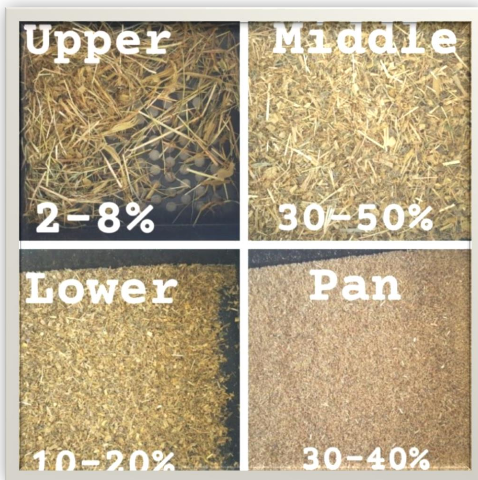
Photograph — the four PSPS fractions (upper, middle, lower, pan) from the author's own sample analysis, with the Penn State Extension-recommended range for each. Author's own photograph.
