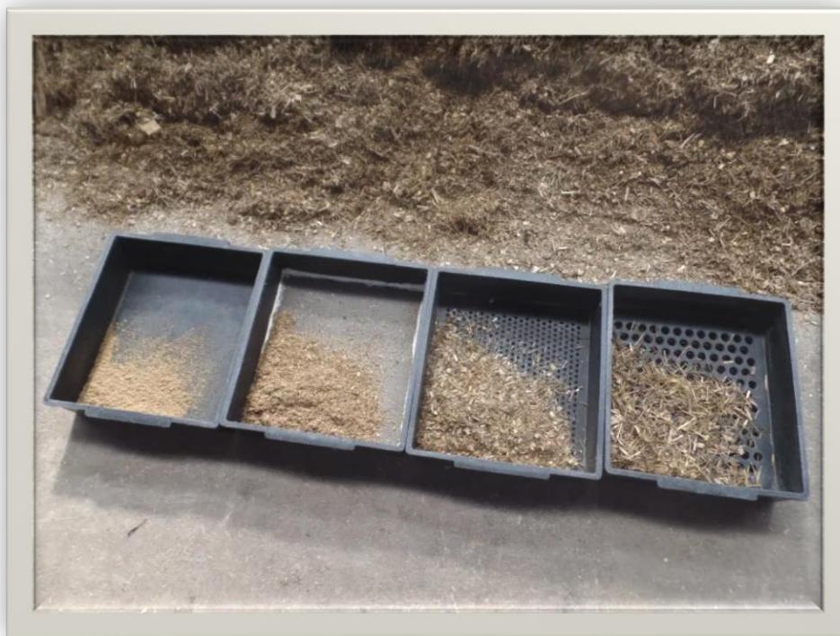
Photograph — a completed PSPS sample showing all four fractions together (pan, lower, middle, upper, left to right). Author's own photograph.
