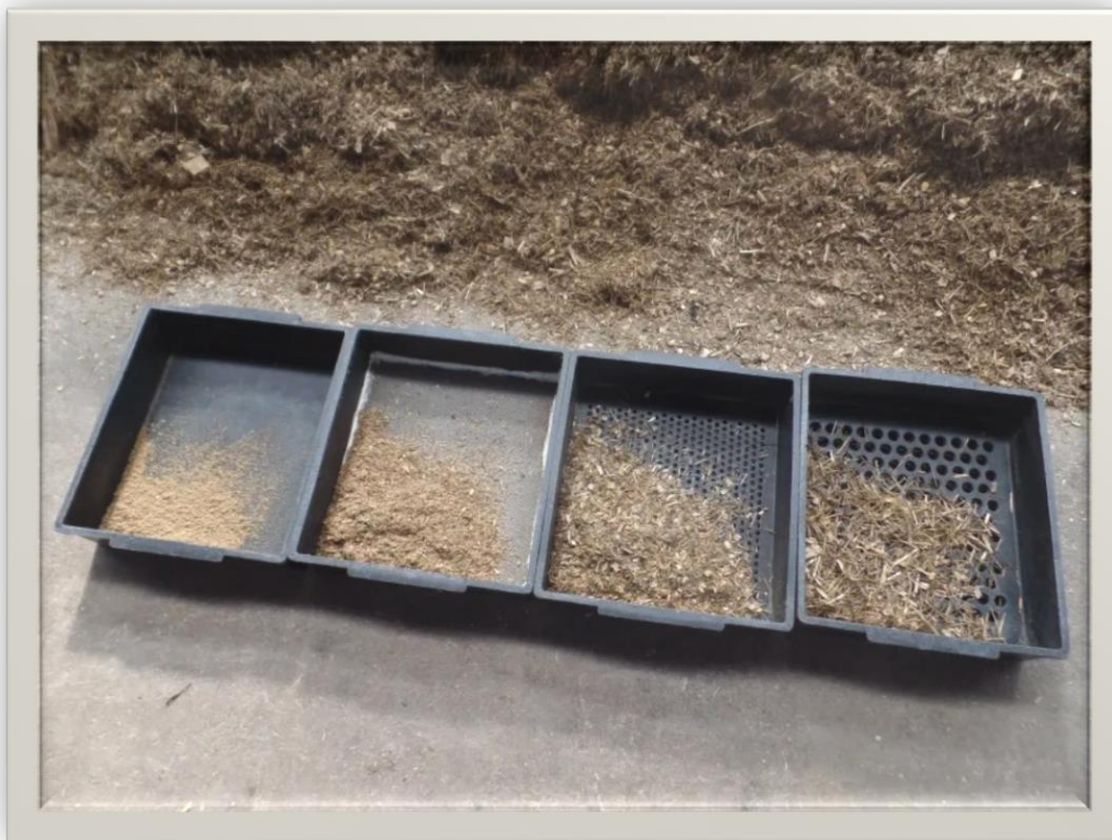
Photograph — a completed Penn State Particle Separator sample, fractionated left to right into pan, lower (4 mm), middle (8 mm) and upper (19 mm) sieve portions..
